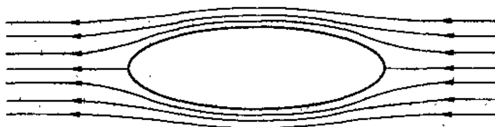
Figure 8.2 Streamline flow around elliptical body
